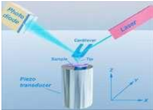
Figure 1. Schematic diagram of an atomic force microscope.
