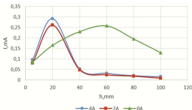
Figure 5. Longitudinal depending of fast electrons concentration on probe in the glow discharge with hollow cathode in the magnetic field.
