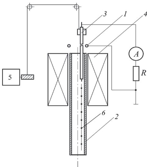
Fig. 1. Scheme of the probe measurements: 1 - anode; 2 - hollow cathode; 3 - electric probe; 4 - electromagnet; 5 - engine; 6 - measurement trajectory.
