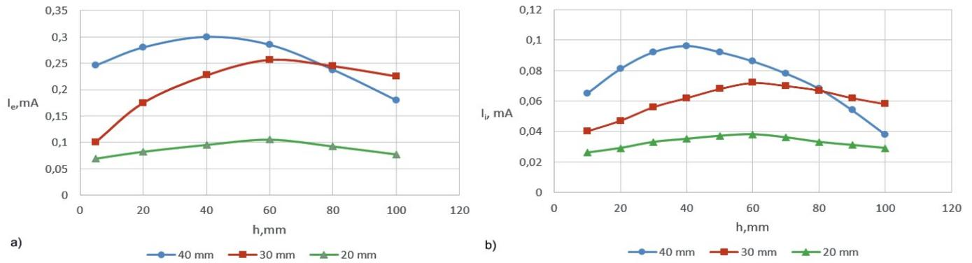
Figure 3. The results of probe measurements: the electron current (a), the ion current (b) for cathode-anode distance  $L_{c-a} = 20$  mm, 30 mm and 40 mm.
