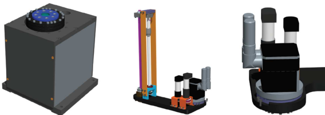
Fig. 6. Engineers proposal of base, support of ballscrew shaft and second axis drive
