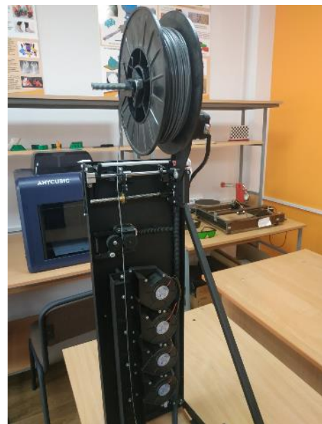
Fig. 2 – Systems of cooling and winding of polymer thread
