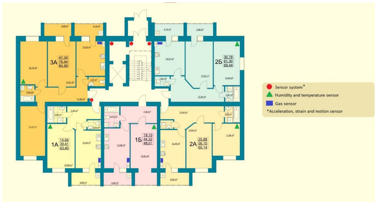
Fig. 1. Diagram of the arrangement of sensors on one of the floors of a residential building
