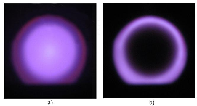
Figure 6. The influence of an external magnetic field at the existence of hollow cathode effect: a) no magnetic field - the effect is observed; b) a magnetic field - no effect.
