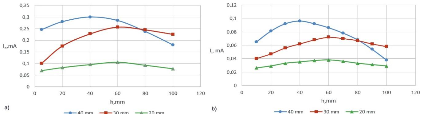
Figure 3. The results of probe measurements: the electron current (a), the ion current (b) for cathode-anode distance  $L_c-a = 20\text{mm}$ ,  $30\text{mm}$  and  $40\text{mm}$ .
