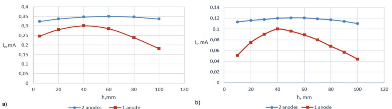
Figure 4. The results of probe measurements: the electron current (a), the ion current (b) with additional anode in the discharge system.
