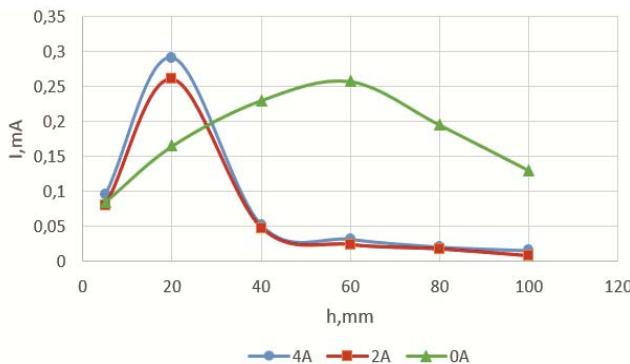
Figure 5. Longitudinal dependence of fast electrons concentration on probe in the glow discharge with hollow cathode in the magnetic field.
