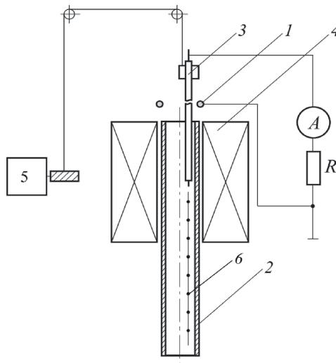
Fig. 1. Scheme of the probe measurements: 1 - anode; 2 - hollow cathode; 3 - electric probe; 4 - electromagnet; 5 - engine; 6 - measurement trajectory.
