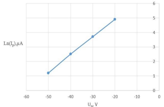
Fig. 2. Current-voltage characteristics of plasma area in a semi-logarithmic scale, in a distance of 20 mm inside the cathode when probe potential changing within the -20 to -100 V, argon pressure  $P = 53$  Pa.
