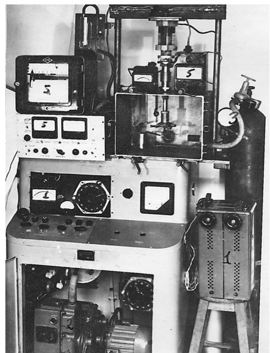
Fig. 3. Kotelnikov's first installation of semi-industrial type for welding in the glow discharge [12].
