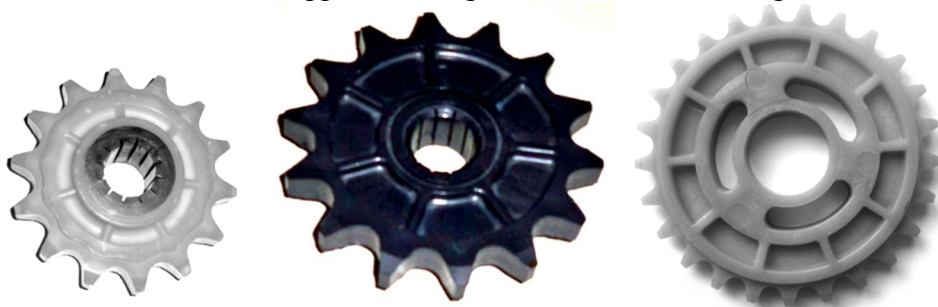
Fig. 10. Tension sprockets of different constructions with separation of heat stream
